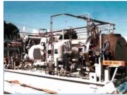
Expander-generator direct drive.
